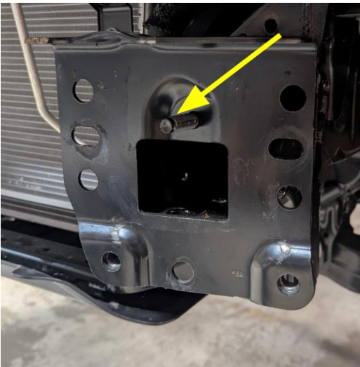
Figure 52 – Mounting Bracket and Weld Stud
