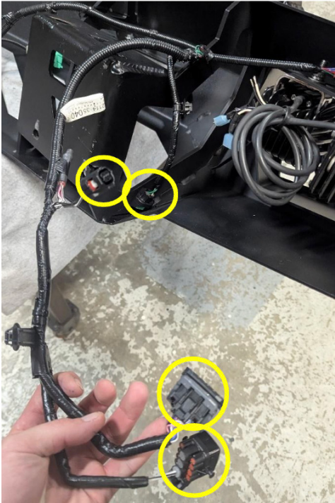
Figure 54 – Wiring Harness Connectors
