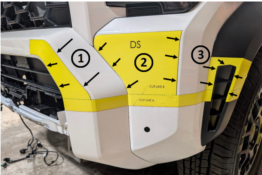
Figure 36 – Template Placement and Sequence
