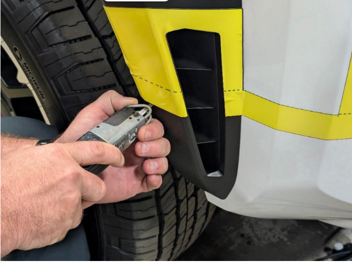
Figure 39 – Trimming Wheel Flare with Template
