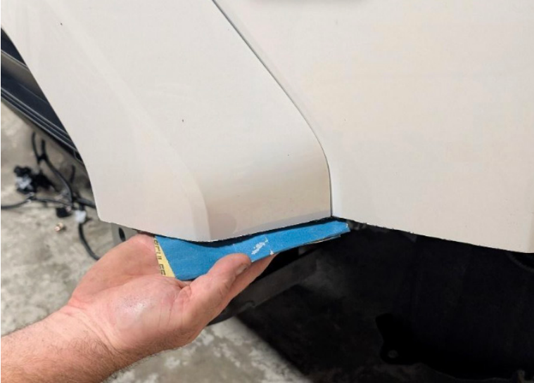
Figure 43 – Burr Removal/Post-Cut Detailing
