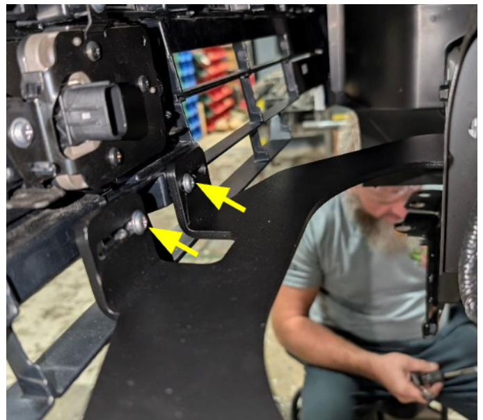
Figure 45 – Grill Support Bracket
