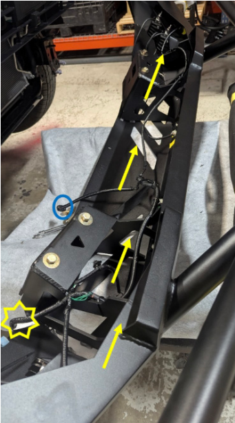
Figure 51 – Wiring Harness Routing
