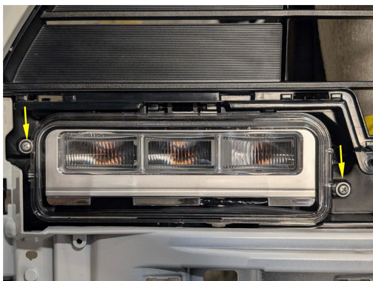
Figure 35 – Fog Light Removal
