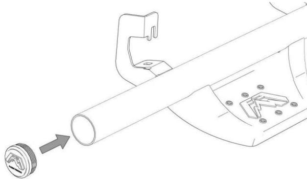
Figure 2 - INSTALLING THE FABFOURS SIDE STEP END CAPS
