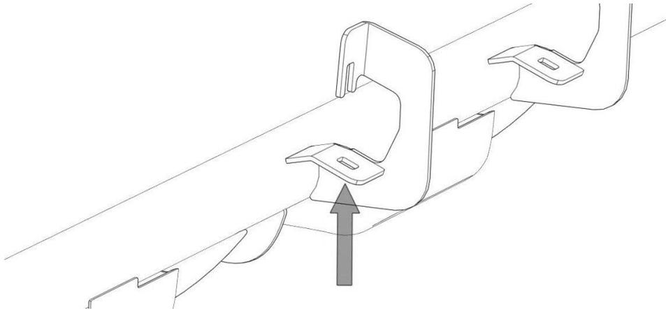
Figure 7 - HORIZONTAL BOLTS INSTALLED THROUGH THESE BRACKET HOLES
