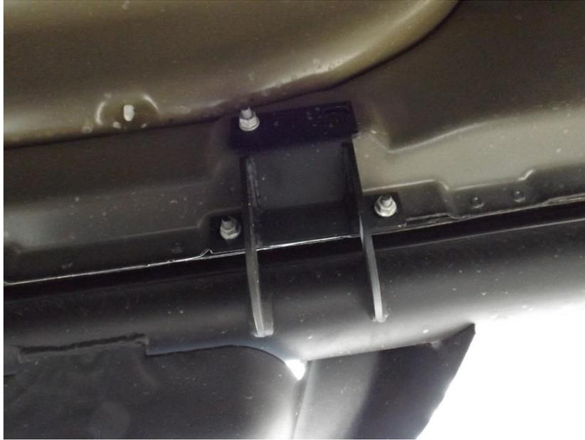
3. With the step in place, thread the M8 flange nut on the three bolts located on truck. Do not tighten.
