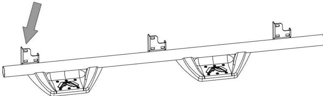
Figure 5 - ADD FRONT 5/16-18 BOLT TO HOLD STEP FIRST
