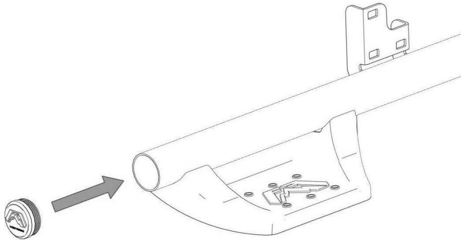
Figure 2 - INSTALLING THE FABFOURS SIDE STEP END CAPS
